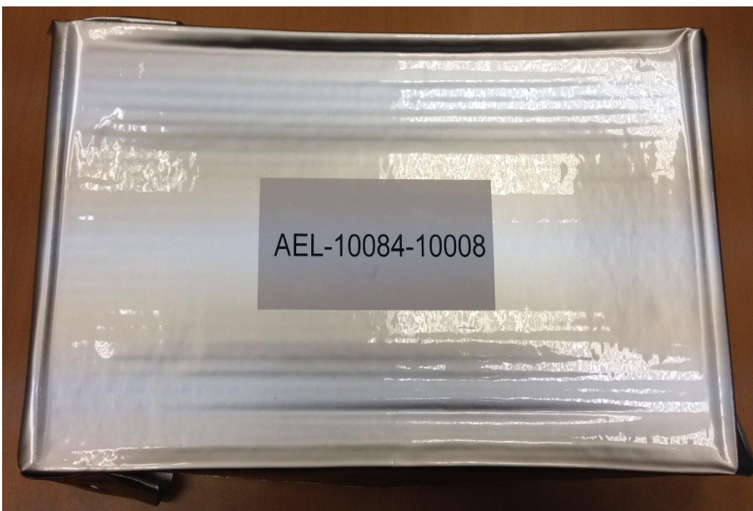
Fig.16 Vacuumed and sealed small carton.
