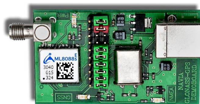
Fig. 3. The Demo Board for the navigation module ML8088sE.
